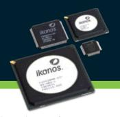
The Fx<sup>™</sup>100100-5 and Fx10050-5 chipsets are the industry's first IPTV-optimized multi-mode (VDSL2,VDSL, ADSL2+, ADSL2 and ADSL) solutions for central office (CO) equipment (DSLAMs,ONUs and other broadband concentrators). Both chipsets support all 8, 12 and 17 MHz profiles. The Fx100100-5 chipset additionally supports the 30 MHz profile. The chipsets also support the VDSL, ADSL2+, ADSL2 and ADSL standards.
