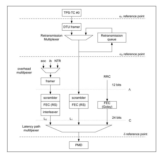
Figure 6: G.998.4 Reference Model (Including Retransmission)
