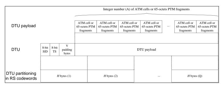
Figure 5 details the various elements of a DTU, where:
