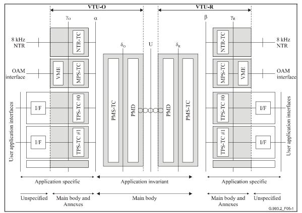
Figure 4: Reference Model for DSL Transceiver: Interfaces and Functional Layers
