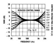
TL/H/5142-7 FIGURE 4. Tone Characteristic (Gain vs Frequency)
