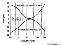
FIGURE 15. Tone Characteristic (Gain vs Frequency)
