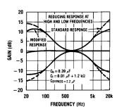
TL/H/5142-9 FIGURE 6. Tone Characteristic (Gain vs Frequency)
