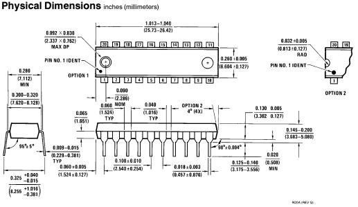
Molded Dual-In-Line Package (N) Order Number LM1036N NS Package Number N20A
