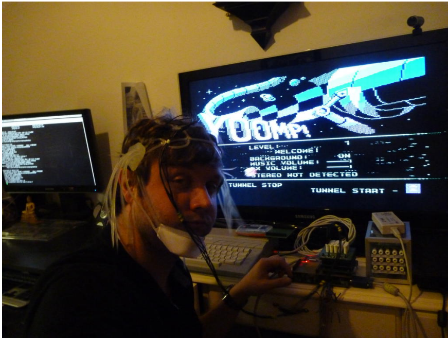
Figure 2.29: CeDeROM BCI FPGA acting as (Atari) videogame controller.
