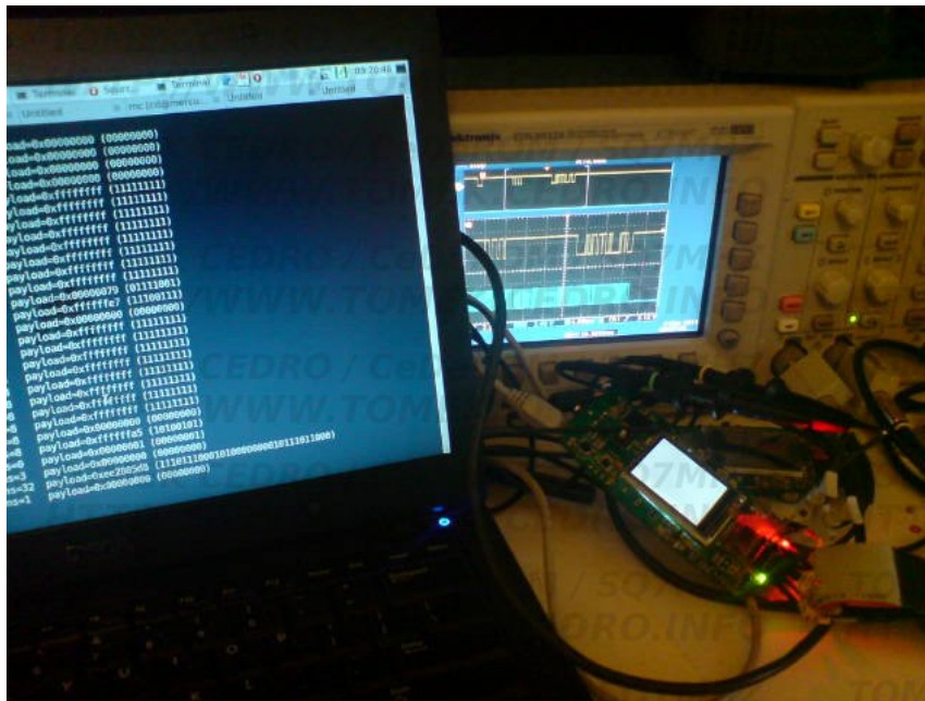
Figure 1.19: LibSWD communicating with Stm32Primer2 using UrJTAG drivers.
